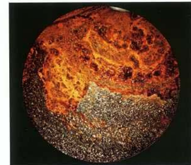
Rust in a car door
