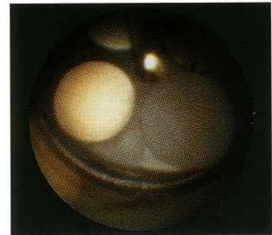
Outlet and inlet valves of a 4-valve engine
