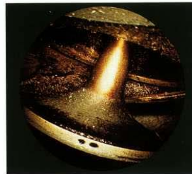
Valve trough through a spark plug socket
